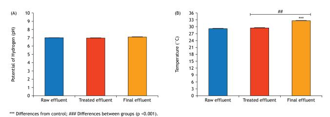
Figure 2. Determination of the potential of hydrogen (A) and temperature (B) of pig farming effluent samples before and after treatment with TEVAP. The results are the mean of independent experiments (n = 3) performed in triplicate.
