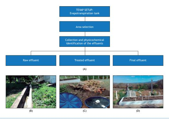
**Figure 1.** Study development flowchart. Sampling locations are indicated: (A) TEVAP setup flowchart and its respective collection phases for analysis; (B) channel through which the effluent flows after pig pen wash; (C) settling box that temporarily receives pig manure before being stored in the TEVAP; and (D) TEVAP - overlapping culture septic basin, germinated after evapotranspiration.
