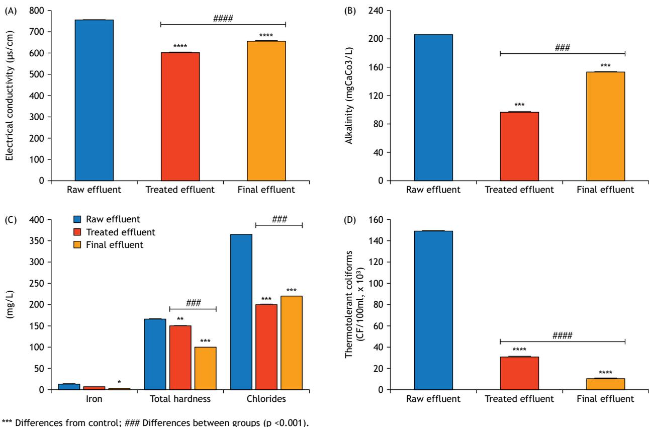
**Figure 5.** (A) Determination of hydraulic conductivity, (B) alkalinity, (C) iron, total hardness and chlorides and (D) thermotolerant coliforms from pig farming effluent samples before and after treatment with TEVAP. The results are the mean of independent experiments ( $n = 3$ ) performed in triplicate.
