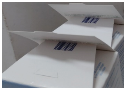
Figure 3: Broken seal or failed glue on secondary packaging.
