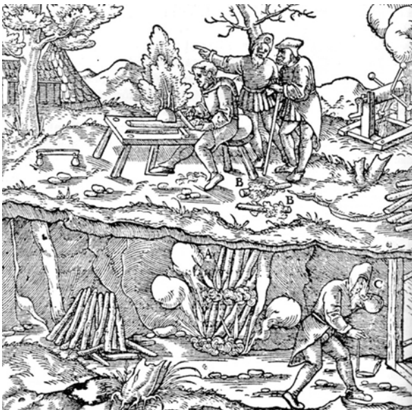
Figure 1. Illustration from the book “De Re Metallica,” one of the first treatises on mining and metallurgy, published in 1550, with detailed information on the risks of death and suffocation and on the health of workers in underground mines, where miners would use fire obtained through the burning of wood for the explosion of mineral shafts and rocks 5 .
