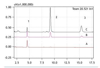
**Figure 5.** Tocopherol profile of samples of vegetable oils. A) Authentic olive oil, B) Commercial oil labeled as olive oil and C) Soybean oil. 1. Alpha-tocopherol. 2. Gamma-tocopherol. 3. Delta-tocopherol.
