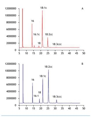
Figure 3. Profile of fatty acids: A) authentic olive oil; B) soybean oil
